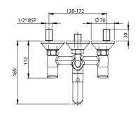
Wall mixer 3-in-1 with provisions for both overhead shower & telephonic shower with 190 mm long bend pipe & wall flange
