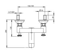
for overhead shower with 160 mm long bend pipe & wall flange
